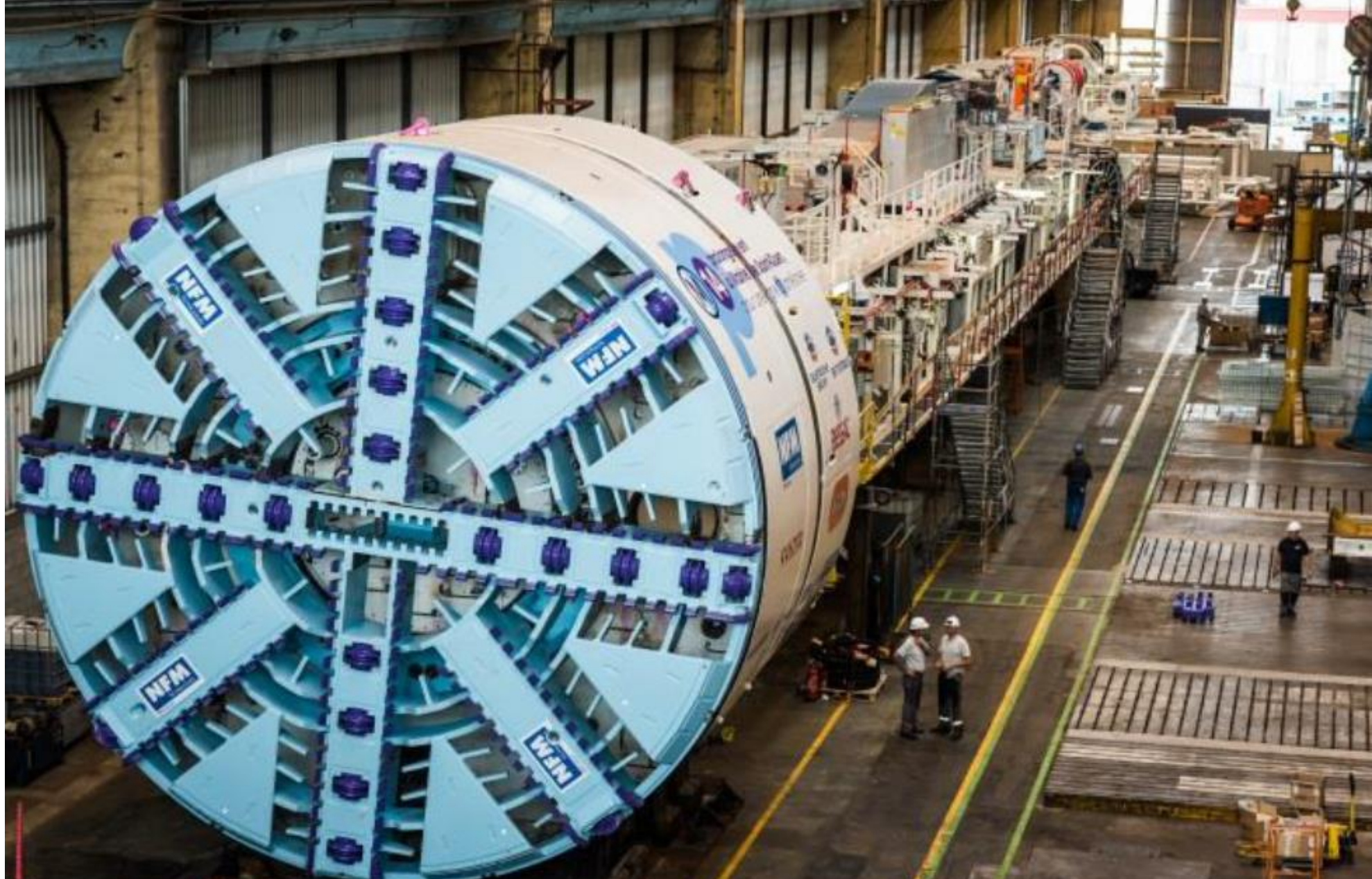
Example Tunnel Boring Machine representative of what would be used to mine the Hudson River Tunnel
